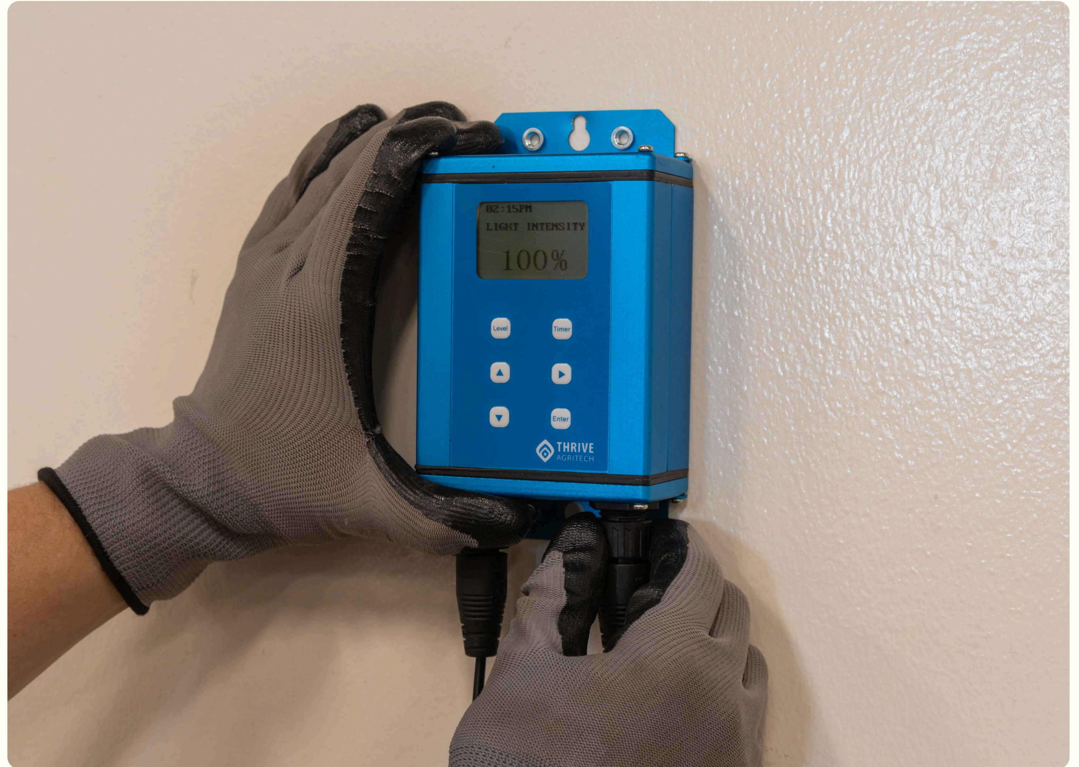
Figure 9. Quick Connect Dimming Cable connection to Dimming Controller box
