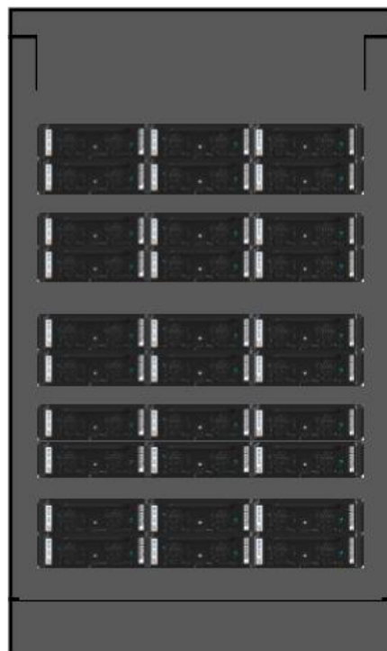
Recommended racking of PDS12 shelves in RK1833BKM Server Rack Cabinet
